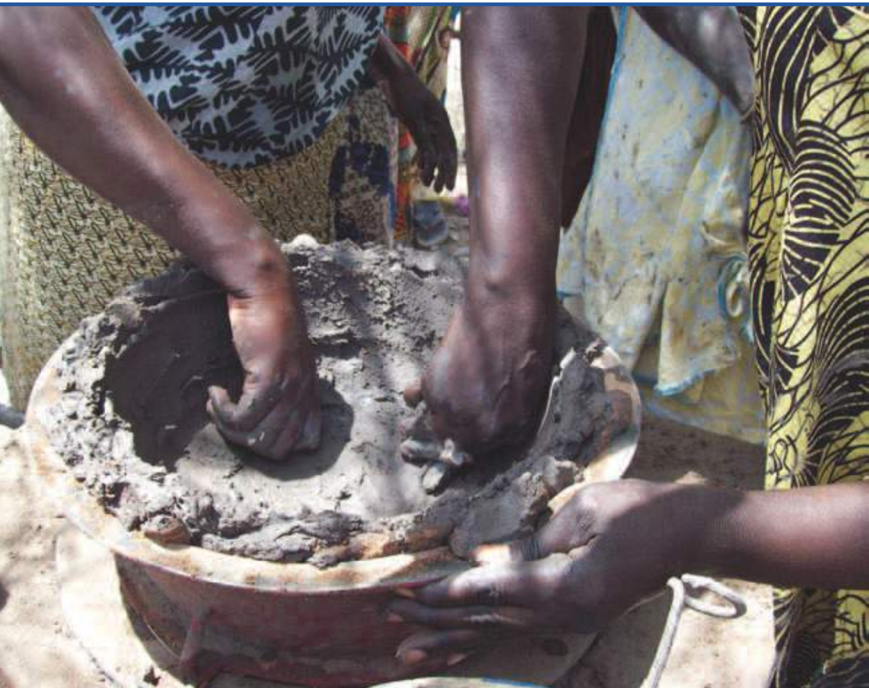
Female stove entrepreneurs in Senegal are moulding clay to produce ceramic stove inserts
