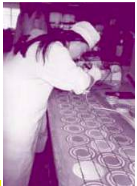
Women in China soldering contacts to PV cells for assembly into PV modules. (Photo: Courtesy of Enno Heijndermans)
